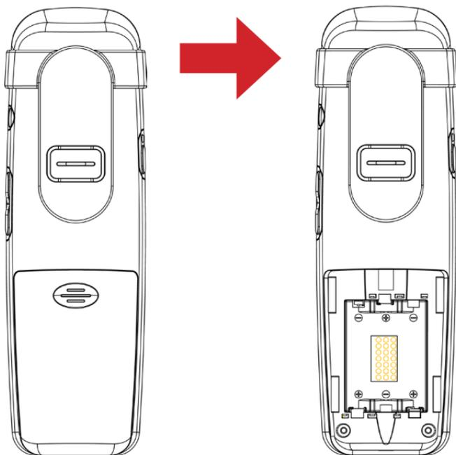
1. Slide back the battery cover and remove the cover.
