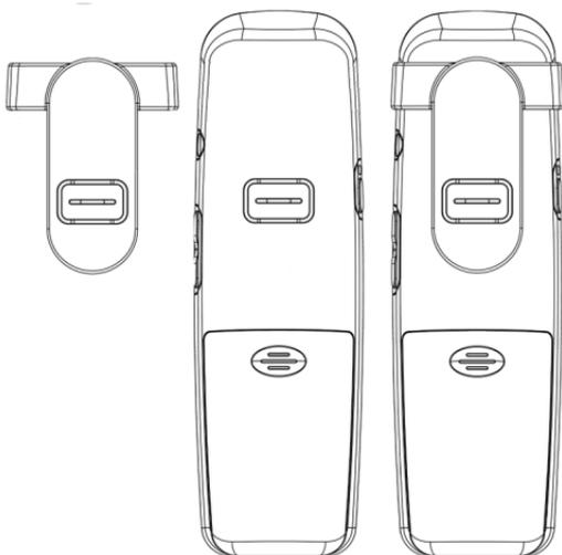
1. On the back of the phone, align the arms of the carrying clip above the slots on the sides of the phone.
